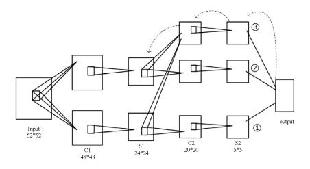
Fig. 3. The first round of growth: the network 'Net1'
