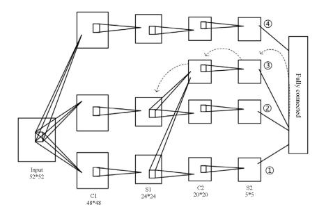
Fig. 4. The second round of growth: the network 'Net2'
